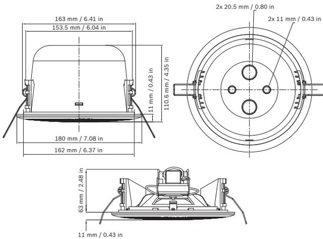
Mechanical diagram LC3-UC06E and LC3-CBB
