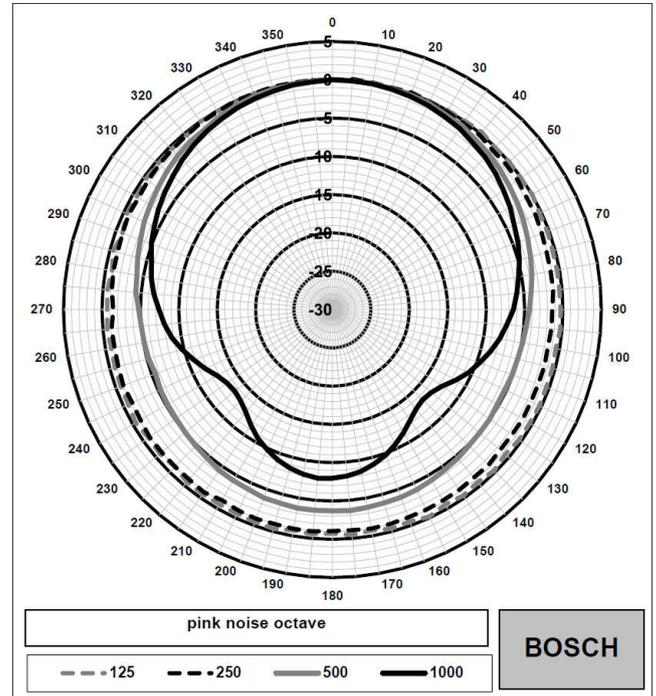
LB2 UC30 Polar diagram horizontal (low frequency).
