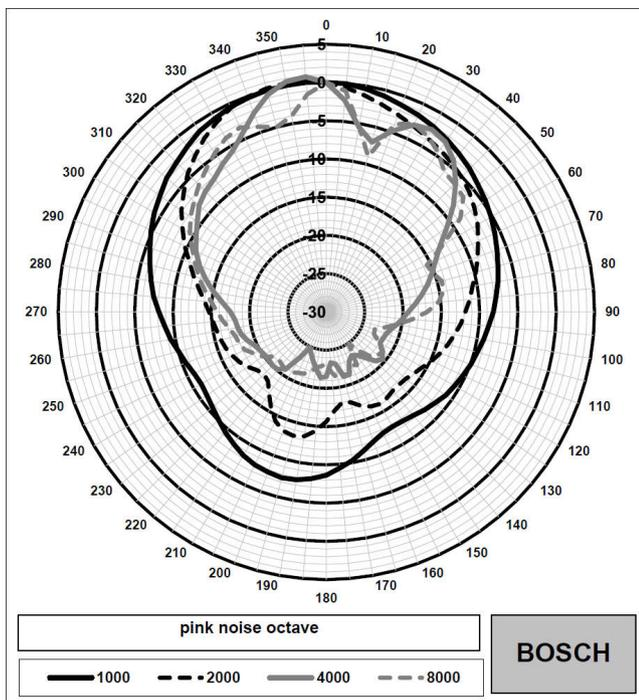
LB2 UC30 Polar diagram vertical (high frequency).
