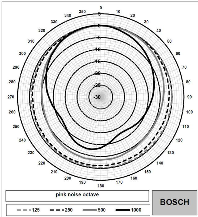
LB2 UC30 Polar diagram vertical (low frequency).
