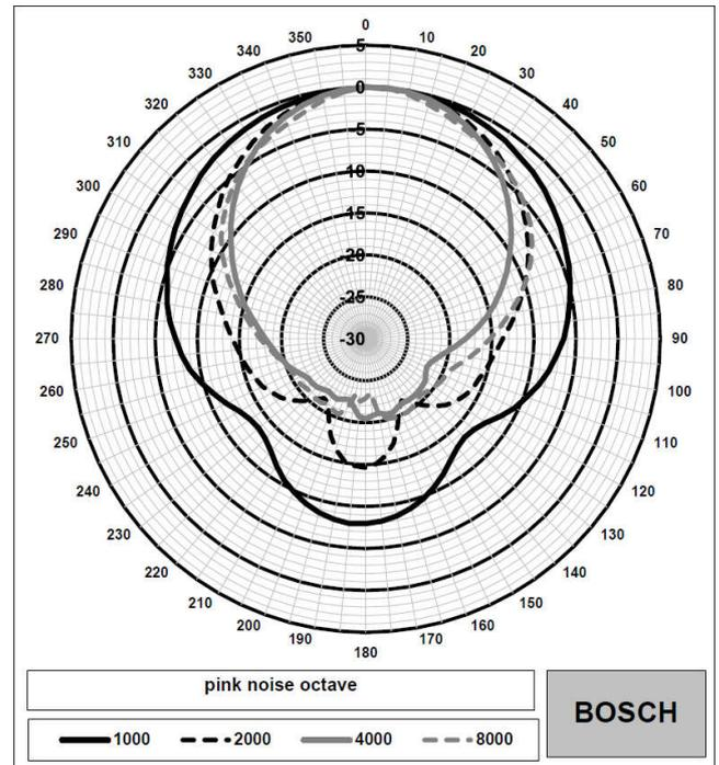
LB2 UC30 Polar diagram horizontal (high frequency).
