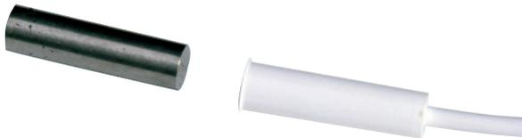
The LSN built-in magnetic contact is used for release monitoring of doors and windows. The contact is tamper-supervised. If an external magnet comes close, the tamper contact is activated and causes a report. Head-on flush mounting.
