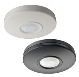
The ceiling mount, low profile panoramic DS936 PIR Detector uses alternate polarity pulse count. It also uses a Fresnel lens to provide up to 7.5 m (24 ft) of coverage and can be mounted on the surface, or semi-flush directly to a ceiling or a standard octagonal electrical box.
