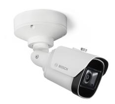
The NBE-3703-AL is a versatile device for general outdoor surveillance monitoring. The compact design for discreet use with quick set-up offers high installation flexibility. The camera offers a 1/2.7" sensor and HDR technology at HD 5 MP. Combined with an integrated varifocal lens, the camera provides a sharp and detailed image with flexible field of view. With added IR functionality, the camera is able to function even in scenes where ambient lighting is not always available.
